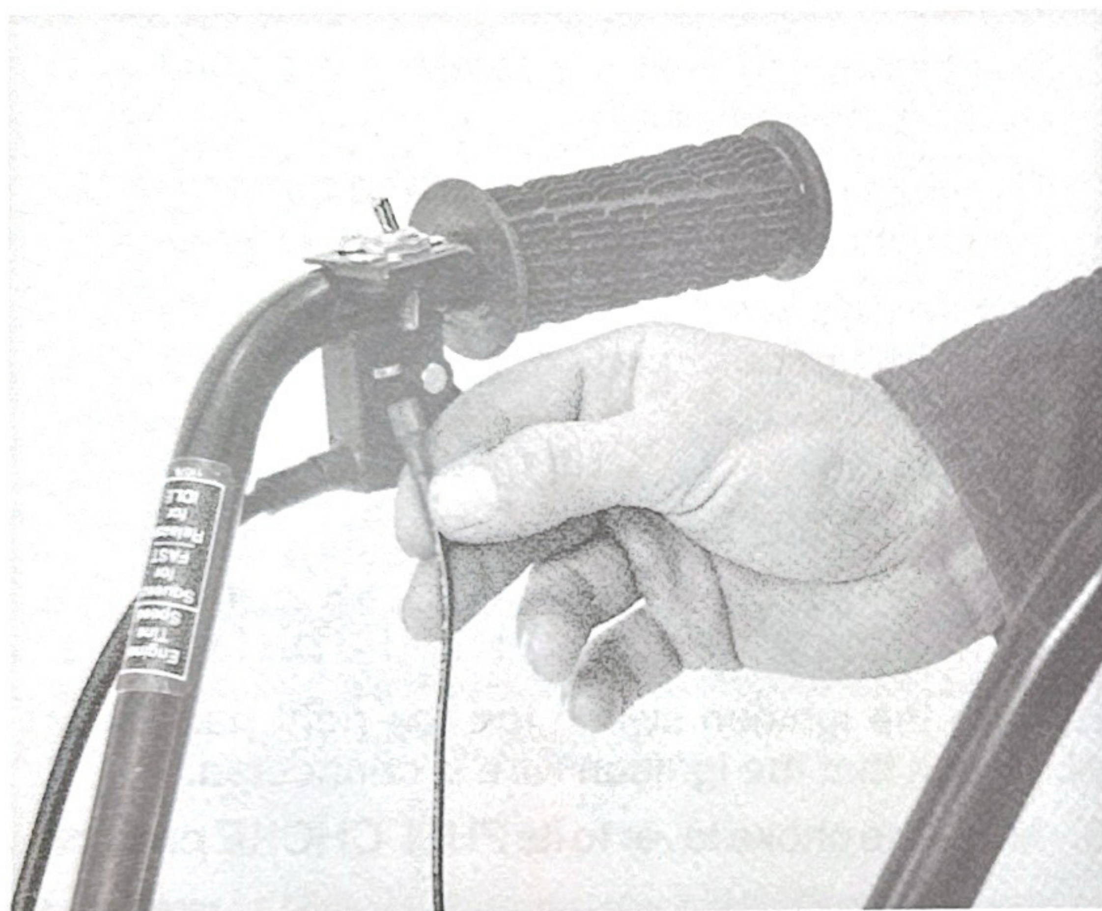
Photo 7: Attaching the On/Off Wire to the Switch
