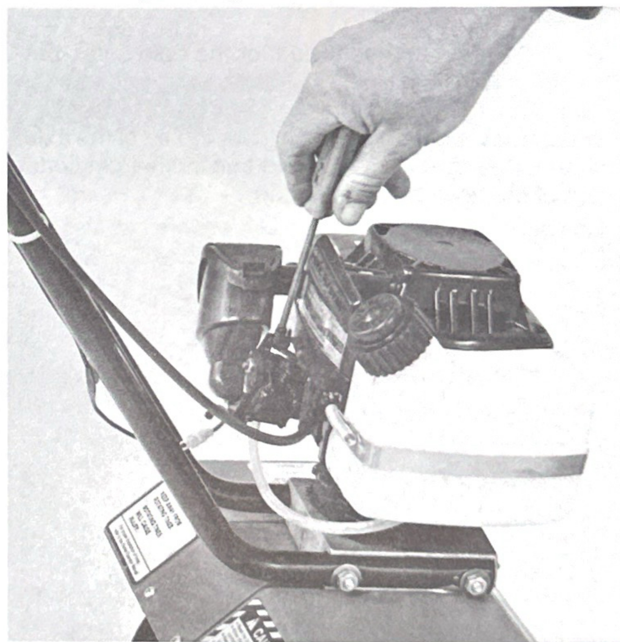
Photo 14: The Carburetor and Its Adjusting Screws
