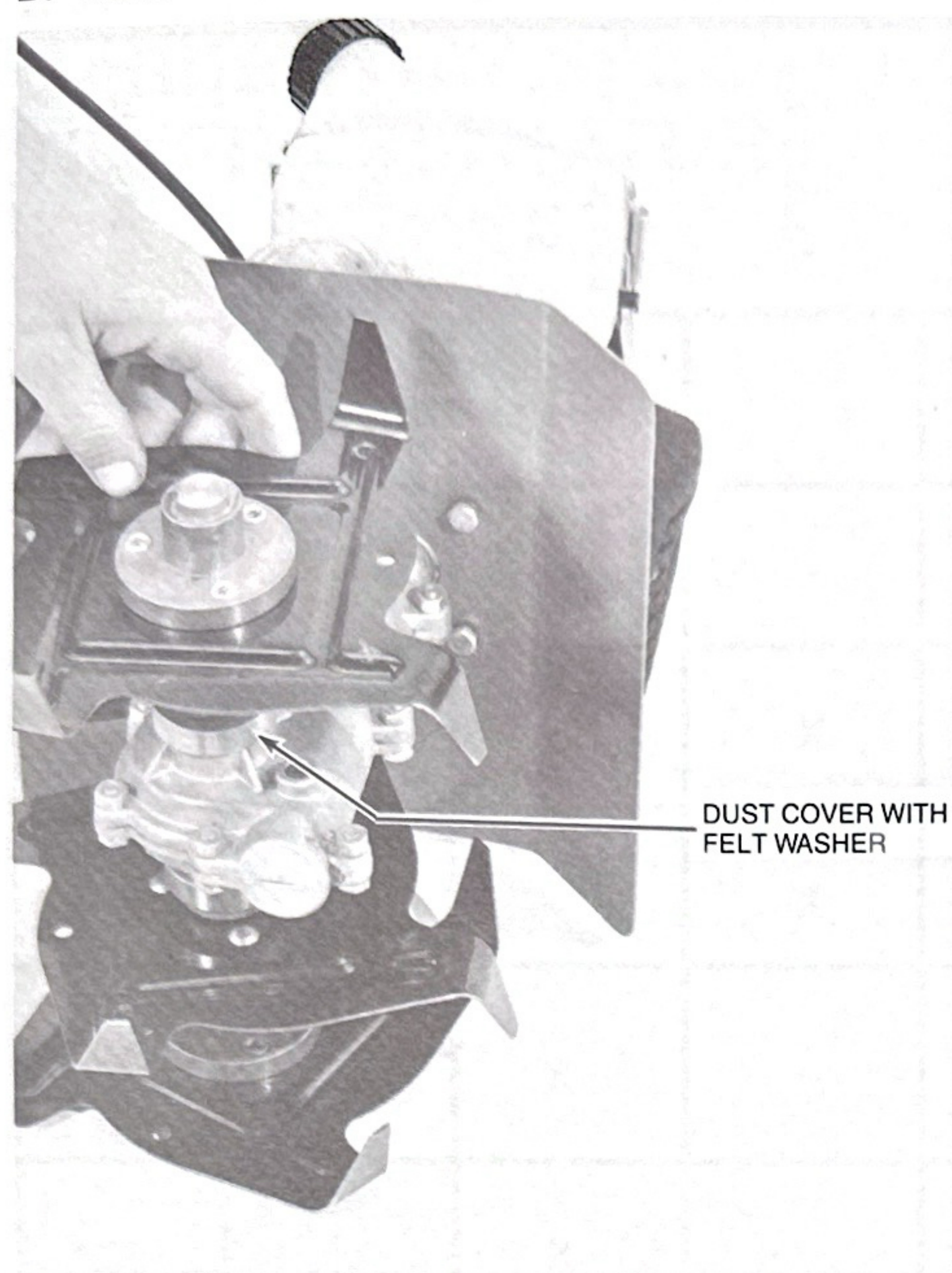
Photo 18: Installing Inner Tine
