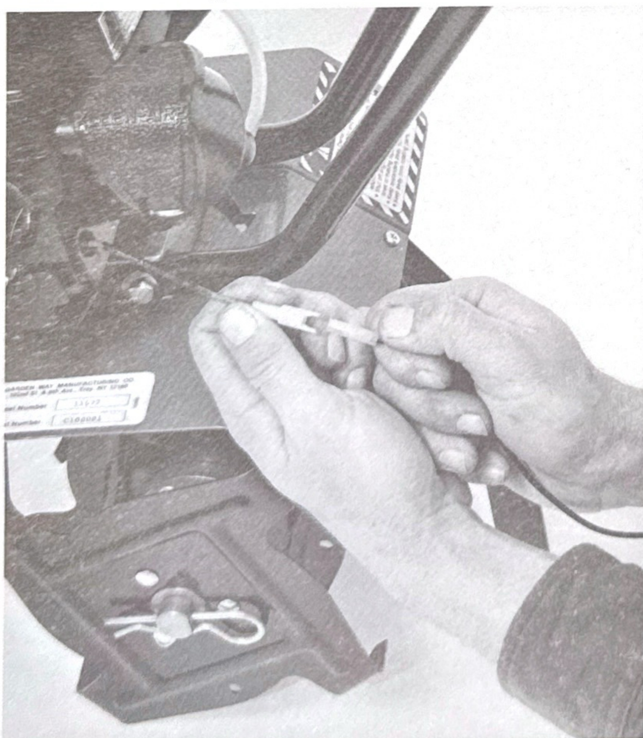
Photo 8: Attaching the On/Off Wire to the Engine
